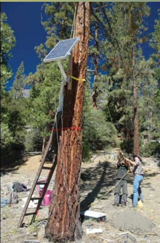
Tree-mounted solar panel being installed at SNEP 54 (Little Yosemite Valley). This station ran through the winter without interruption.
