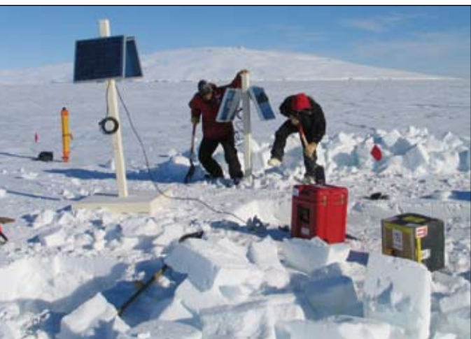
Jonathan Thom and a field assistant deploying a PASSCAL seismometer on the giant tabular iceberg C16 in the Ross Sea, Antarctica, as part of a project to understand the sources and mechanisms of "iceberg tremor" detected as far away as Tahiti and the South Pole.
